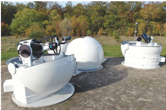
GATS PST3 – modern set of 5 optical telescopes with diameters from 30 to 70 centimeters and field of view from 0.5 to 3.2 degrees, equipped with its own computer cluster and scientific-CMOS type cameras. The set is dedicated to astrometric and photometric monitoring of Earth's artificial satellites and space debris. Credit: AOI AMU
