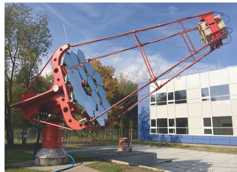
SST-1M Cherenkov telescope prototype on test station at INP PAS, proposed for Cherenkov Telescope Array observatory. Credit: J. Niemiec/INP PAS
