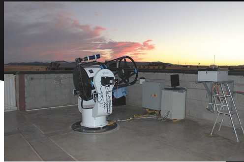
GATS PST3 – modern set of 5 optical telescopes with diameters from 30 to 70 centimeters and field of view from 0.5 to 3.2 degrees, equipped with its own computer cluster and scientific-CMOS type cameras. The set is dedicated to astrometric and photometric monitoring of Earth's artificial satellites and space debris. Credit: AOI AMU
