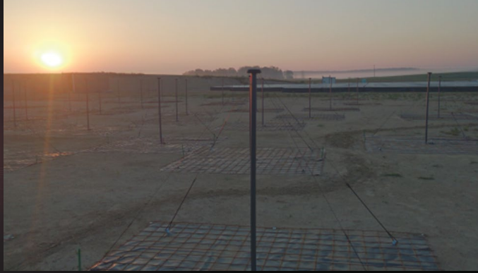
LOFAR radiotelescope antennas. In the foreground: LBA antennas (Low Band), in the background: High Band – HBA. Credit: UWM
