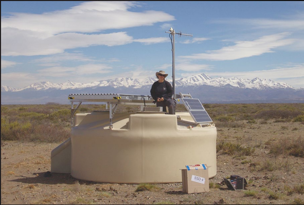
Mounting the SSD scintillation detector on one of the surface detector stations at Pierre Auger Observatory. Credit: Pierre Auger collaboration
